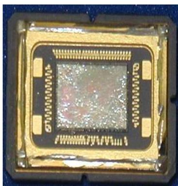
A complete DMA contains 848 columns and 600 rows of mirrors and measures 10.2 mm x 13.6 mm. Here, a DMA is shown with its glass cover removed.
