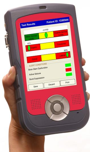
**Fig. 1.** Prototype of portable Brain Stethoscope (BrainScope™) device for use in Emergency Departments (ED). The result of the three-level classification is indicated graphically on horizontal color bars. In addition, the device indicates the result of three alert conditions (BrainStem Dysfunction, Active Seizure, Burst Suppression).
